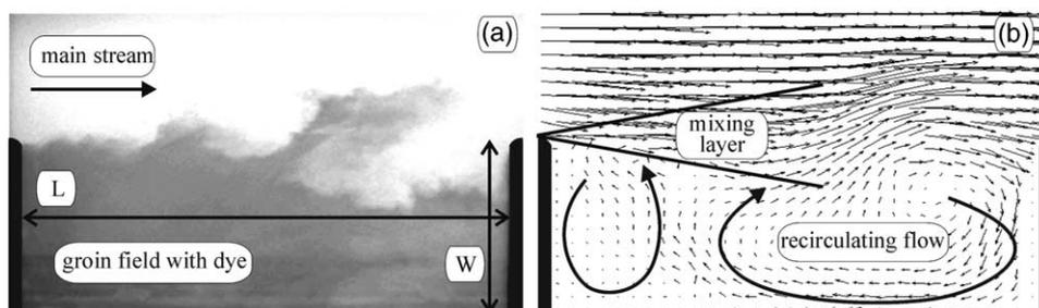
Fig. 8. Flow dynamics in a mixing layer between groin field and main stream, (a) dye experiment, (b) PIV data of an instantaneous velocity field.
