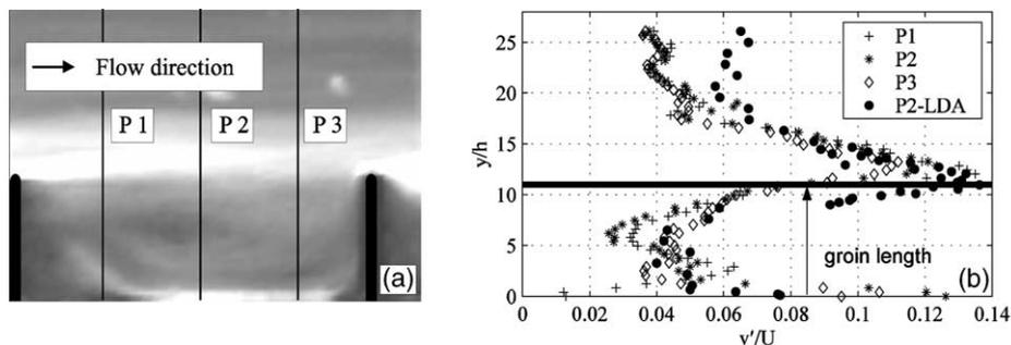
Fig. 10. Turbulent flow characteristics, (a) visualization of the turbulent velocity fluctuations in transverse direction, (b)  $v'$  profiles at 3 different sections of the flow field. The values are normalized by the water depth  $h$  and the main stream velocity  $U$ .
