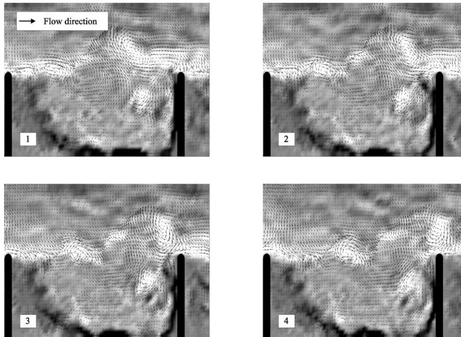
Fig. 11. Series of vorticity fields with time intervals of 1 s. Light color indicates clockwise rotation and dark color anticlockwise rotation.
