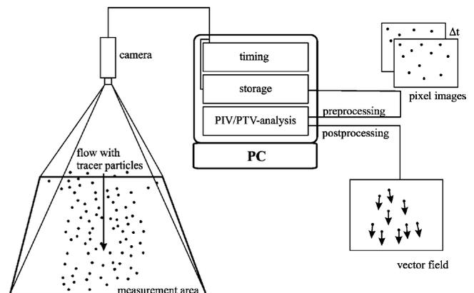
Fig. 1. Schematic sketch of a PIV-system.
