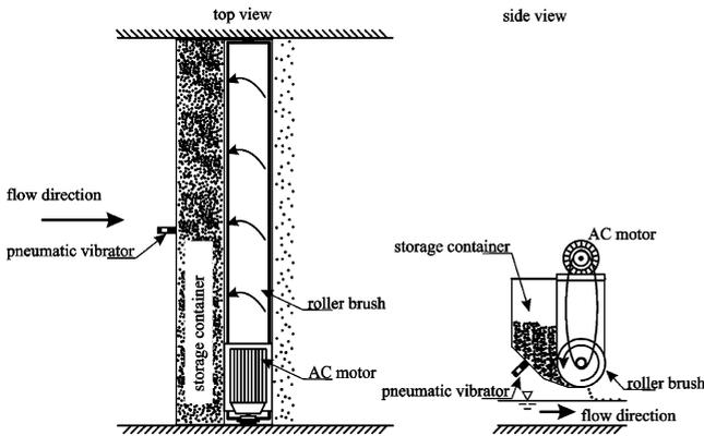
Fig. 2. Schematic sketch of particle dispenser.
