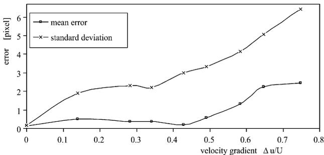
Fig. 5. Accuracy of pixel displacement, related to the velocity gradient in an interrogation area.
