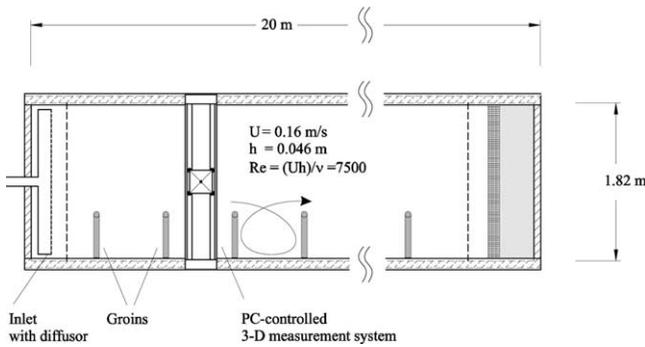
Fig. 7. Schematic sketch of the experimental setup.
