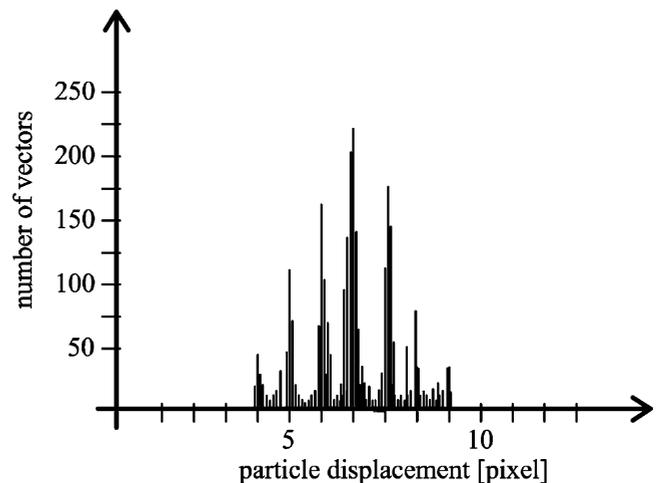
Fig. 3. Illustration of peak locking effect associated with insufficient particle image size, by showing a histogram of PIV displacements.
