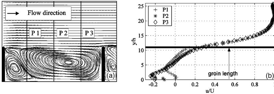
Fig. 9. Mean flow properties, (a) streamlines of flow in the dead-water zone, (b) velocity profiles at 3 different sections of the flow. The velocity profiles are normalized by the water depth  $h$  and the main stream velocity  $U$ .
