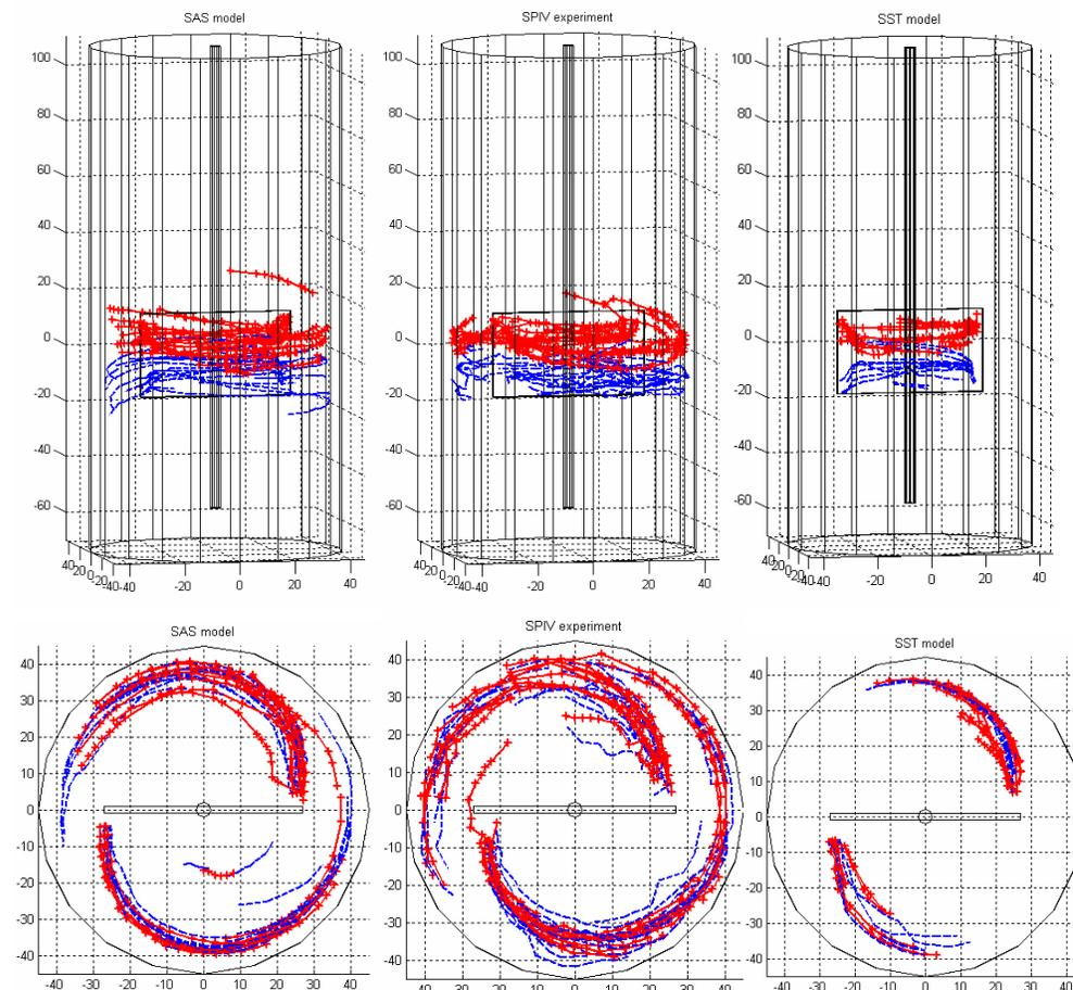
Figure 2. The three-dimensional trajectories of trailing vortices. Left SAS model, middle experimental, right SST model. The upper images show the side view, lower the top view.
