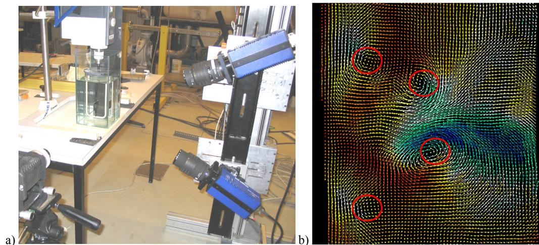
Figure 1. a) Experimental setup and b) an instantaneous 2d-3c velocity field in a turbine discharge zone. Vector colour shows the tangential velocity (red = 0 m/s, blue = 0.4 m/s). Vortices are shown with red circles.
